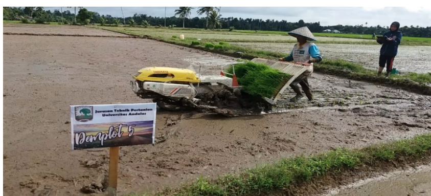
Figure 3. Rice planting process using rice transplanter
